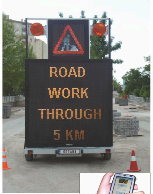
PDA Controlled MVMS PDA Kontrollü MVMS
